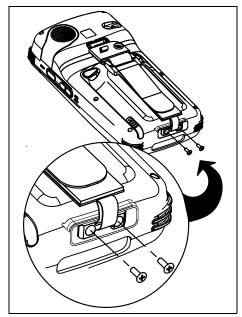
4. Adjust the hand strap by pulling up the Velcro tab and readjusting to your hand as needed.
